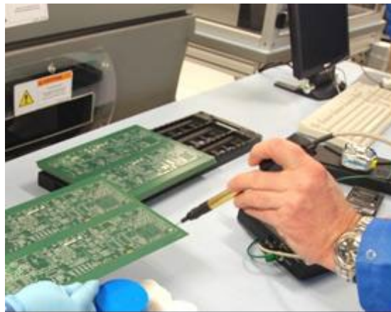
Figure 32 — Measuring PC Conductor with High-Impedance Contact Voltmeter
