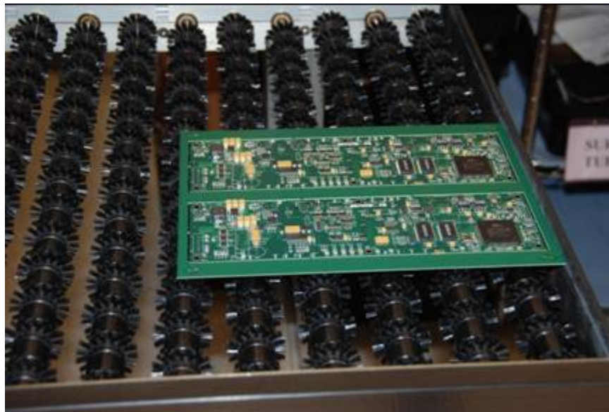
Figure 35 — Uncontrolled Brushes Generate > 500 V on PCBs
